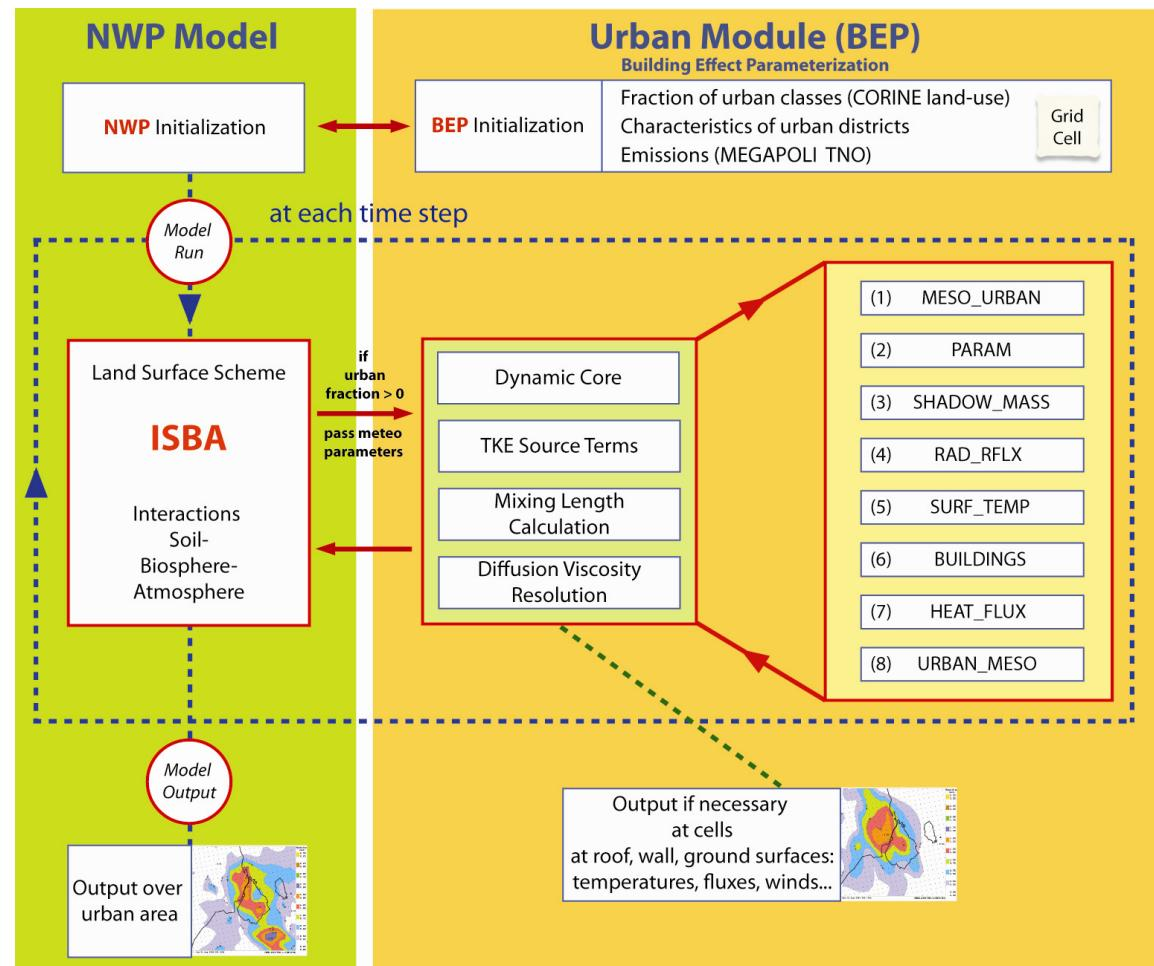
**Figure:** General scheme of the BEP module for the model urbanization with a structure of the subroutine conception.
