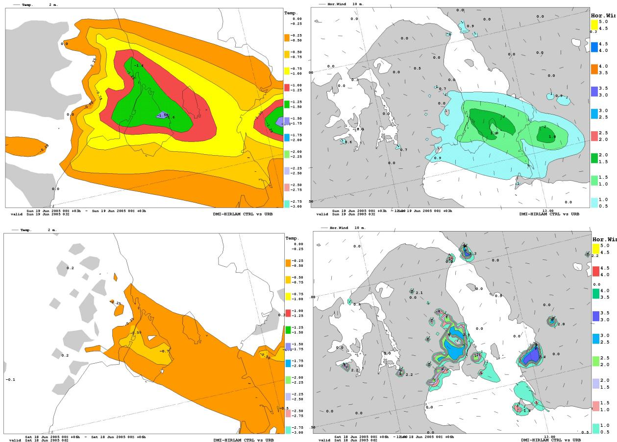
**Figure / Example:** Difference fields between the modified (urbanized: for AHF, R, BEP) and control runs of the model for the air temperature at 2 m and wind speed at 10 m on SELECTED DATE, TIME for the SELECTED metropolitan area.
