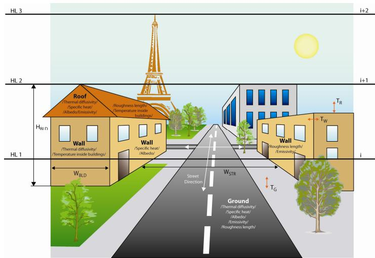
**Figure:** Schematic representation of urban features and numerical grid in the urban module /  $HL1, HL2$  – model levels;  $H_{BLD}$ ,  $W_{BLD}$  – height and width of the buildings;  $SD$ ,  $W_{STR}$  – street direction and width;  $T_G$ ,  $T_W$ ,  $T_R$  – temperatures of ground, wall and roof surfaces, respectively/.
