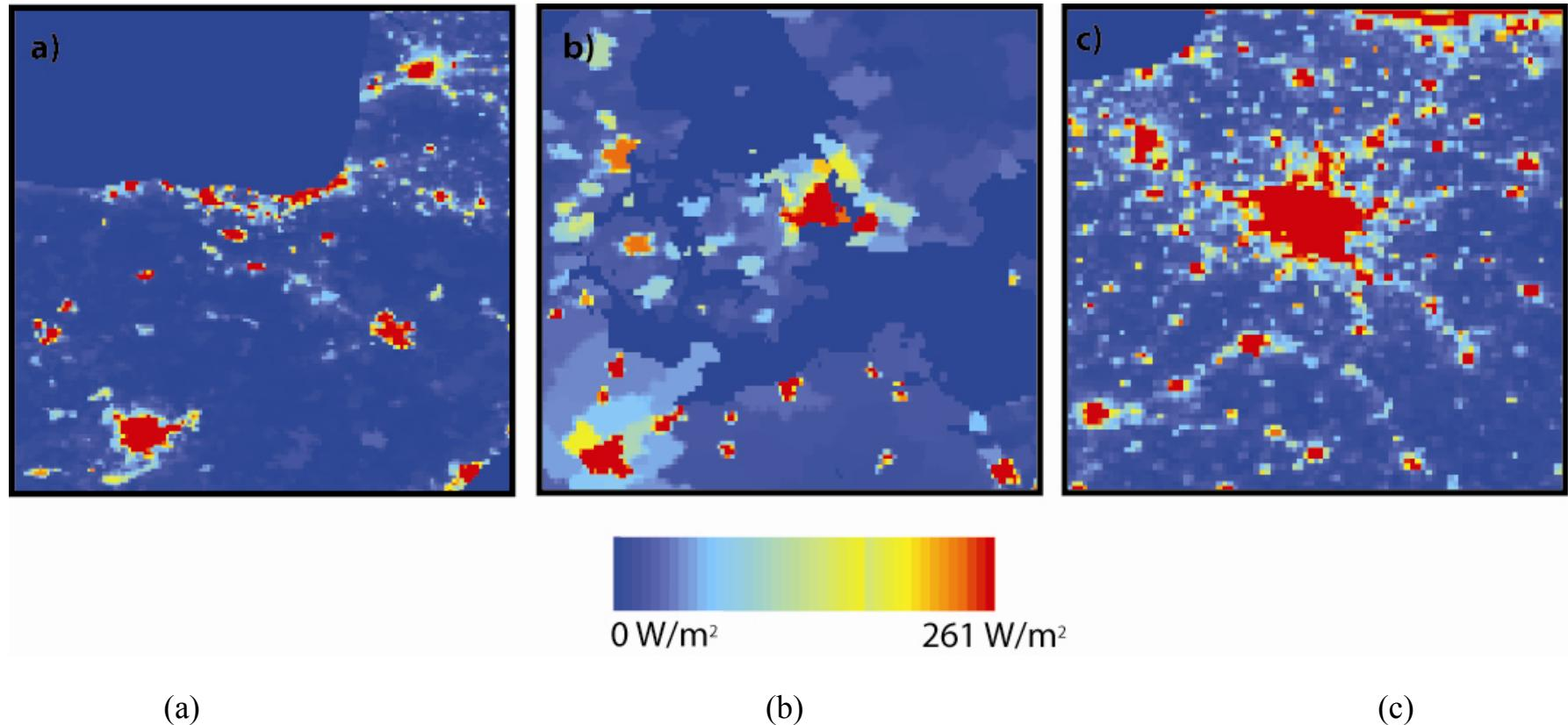
**Figure:** Athropogenic heat fluxes (in  $\text{W/m}^2$ ) for 2005 based on extracted from the LUCY model for the:
